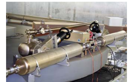
G ring laser after installation of 150 mm vacuum tubes and getter tank (behind wheel valve).
